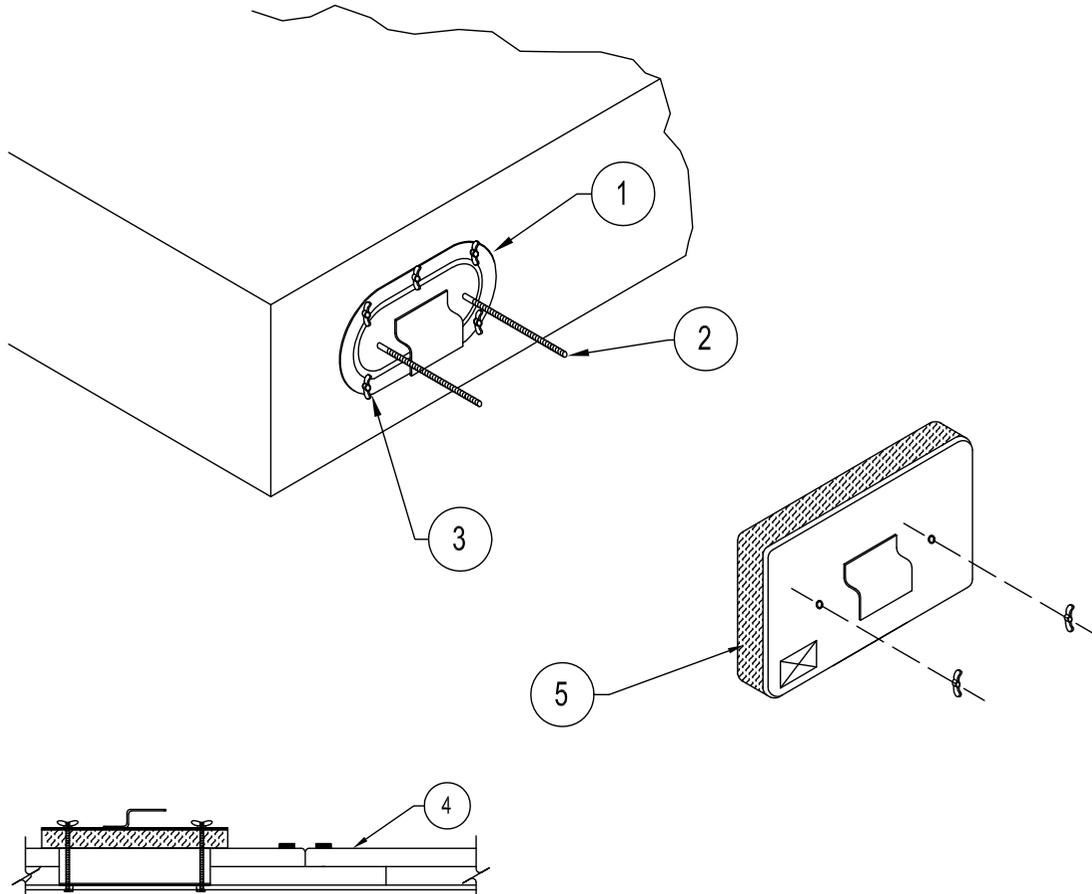
ASTM E 2336 Compliant Enclosure and Door System
