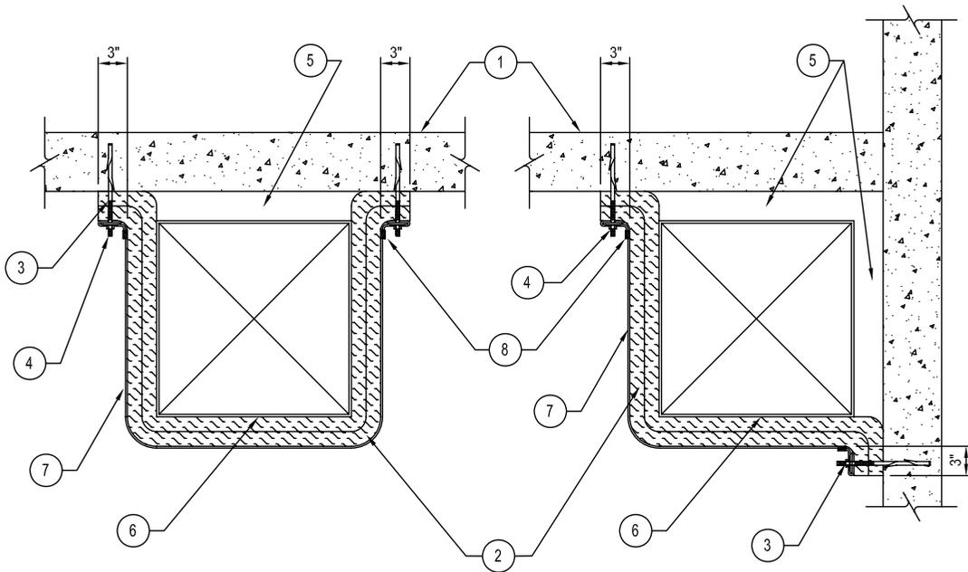
Note: Ducts must be independently supported per code
